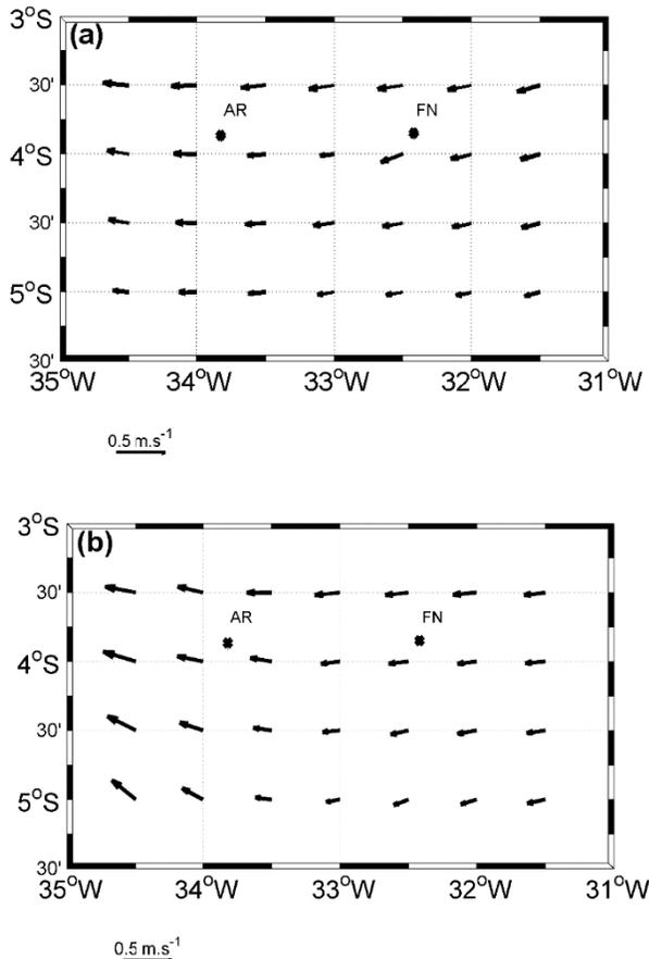
Fig. 3 — Current annual means [m/s] from our ROMS simulation (a) and DRIFTERS (b).
