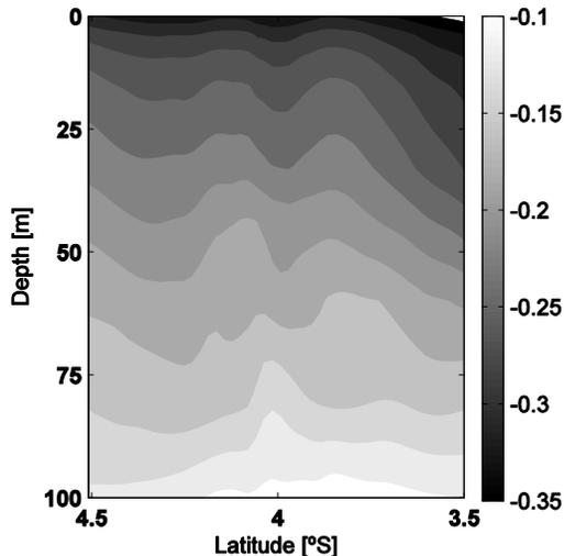
Fig. 9 — Vertical section of the annual mean zonal current [m/s] at 32°W.
